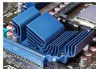
The fins on a heat sink conduct heat away from the chips that are generating the heat.
