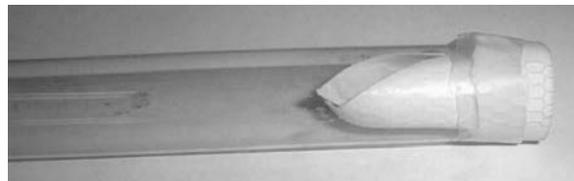
**Figure 1:** This valve was constructed by cutting the finger off a rubber glove, cutting a hole in the fingertip, and taping the glove finger to the end of a plastic tube.
